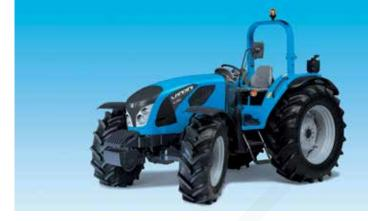
The 5H tractor range from Landini is revamped with the new Perkins 854E-E34TA 3.4L, four-cylinder engines, all featuring a two-valve cylinder head, a common rail injection system, turbocharging and an air-to-air aftercooling system. Equipped with an innovative exhaust gas recirculation system (EGR) which reduces NOx emissions at source, these engines meet the Tier 4 Interim emission regulations without the use of fuel additives.
