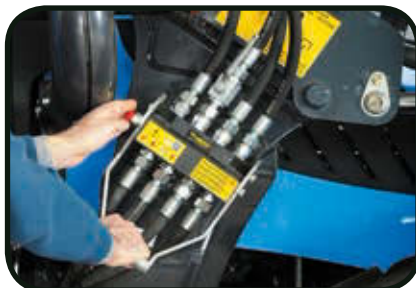
Quick-connect multi-coupler for tractor/loader hydraulic connection
